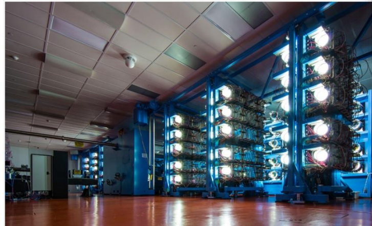
The OMEGA laser's 20-cm disk amplifiers at the University of Rochester's Laboratory for Laser Energetics. (Photo by Adam Fenster/University of Rochester)
