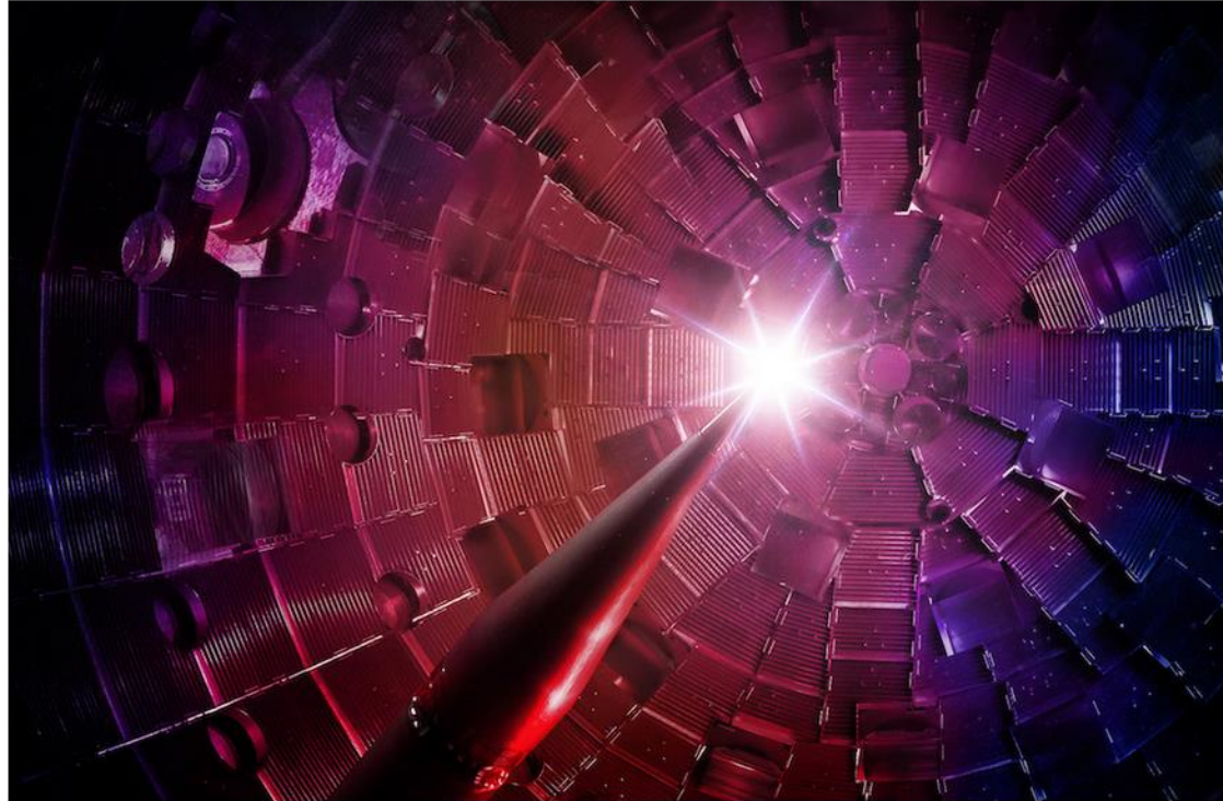
Inside the chamber of the National Ignition Facility, 192 pulses of laser light bombard a target nearly simultaneously. Credit: Lawrence Livermore National Laboratory
